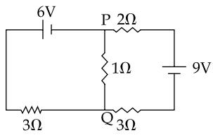
In the circuit shown, the current in the  $1\Omega$  resistor is :
